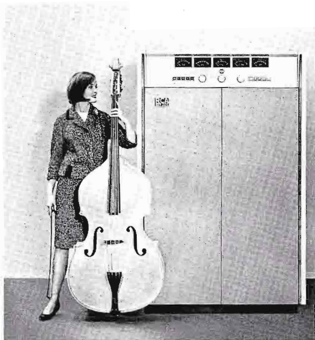
RCA 20-KW FM transmitter has same cabinet as 5-kw and 10-kw.
