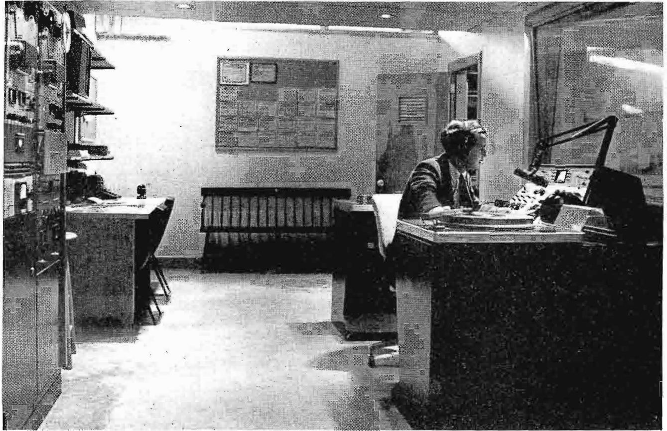
FIG. 2. View of the Control Room shows a student seated at the custom built Master Control Desk with an RCA Audio Console, two turntables, microphone and storage space. The Control Room also contains API Teletype, equipment racks, work table and extra seating to encourage student interest and participation.
